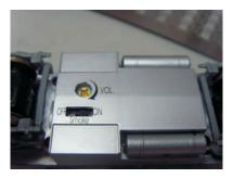
When the output begins to diminish significantly, add 8-10 drops to recharge the unit. Again, give it a few seconds to warm back up. The cool fluid slows the action for a few seconds. Also, watch out for bubbles that may block the stack. You may need to gently blow down the stack to clear it.
