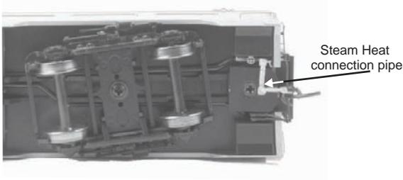
2. Remove the screw on the coupler pocket and remove the coupler from both ends of the car. (Be careful not to damage the coupler release bar.)
