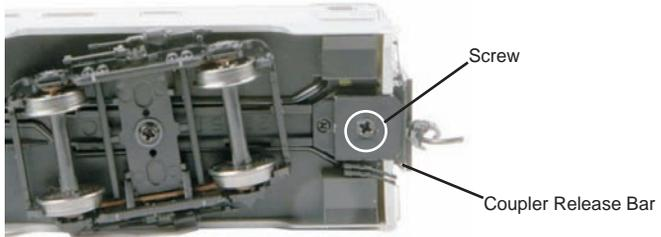
3. Then slightly pull outward on the body near a truck as you pull up on the truck. After you free one side repeat this step on the other end of the car. Gently lift out the interior from the body
