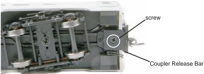
There is a second screw hole behind the hole where the coupler was originally attached. Reassemble the coupler in the second screw hole position.
