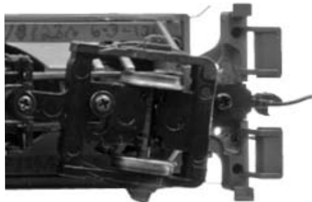
Engine Coupler Installed Underside View
