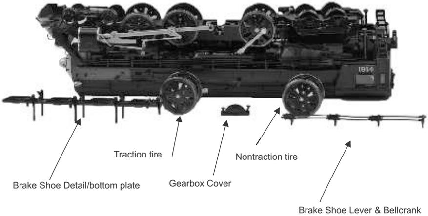
Now, very slowly and carefully lift the wheel set upward. Keep a close eye out for the driver springs as they sometimes stick to the bushings and lift out. If you drop one, you'll need some really good eyes or a magnet to find them. If they should lift out with the wheel set, carefully set them back into cavities from which they came.
