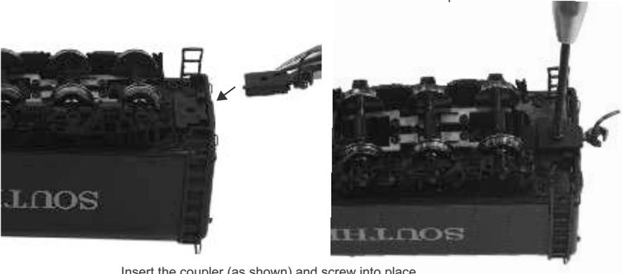
Insert the coupler (as shown) and screw into place
