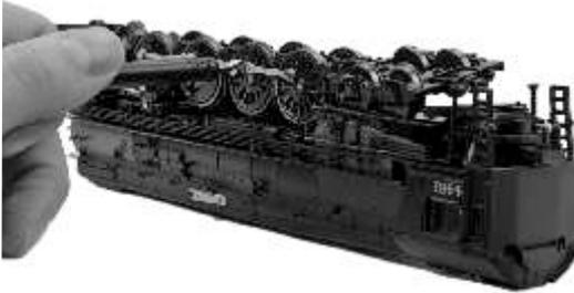
Next, remove brake shoe detail by gently prying and pulling up the part and set aside. Remove the 5 screws holding down the rectangular chassis bottom cover. Carefully remove the cover... then carefully remove the 2 screws holding down the *gearbox* cover, set them aside and then stop. Don't do anything further until reading the next step completely.
