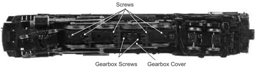
Before proceeding, there are a couple of important things to know. First, under the square bushings on each end of the axle are tiny springs. They are critical to the proper operation of your engine and you don't want to drop them. Next, look closely at the wheel set and bushings and take note of their orientation.
