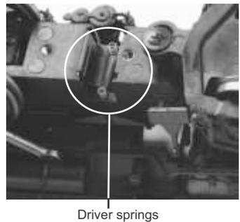
Drop the replacement wheel set into the chassis. Make sure the bushings are in the correct orientation. The small rectangular tabs on the front and rear must be upward (with the engine upside down) toward the chassis bottom cover.
