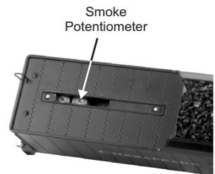
The manual smoke potentiometer under the control hatch (on top of the tender) must be fully clockwise for the F12 key to function. When the smoke potentiometer is fully counterclockwise, the smoke is always off.
