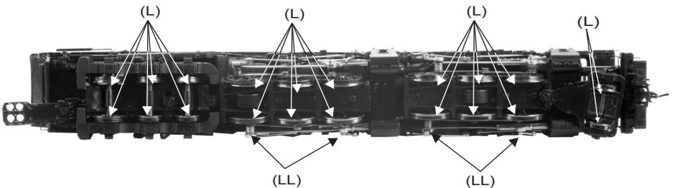
Lubricate Side Rods and Linkage (Both Sides) (LL)
